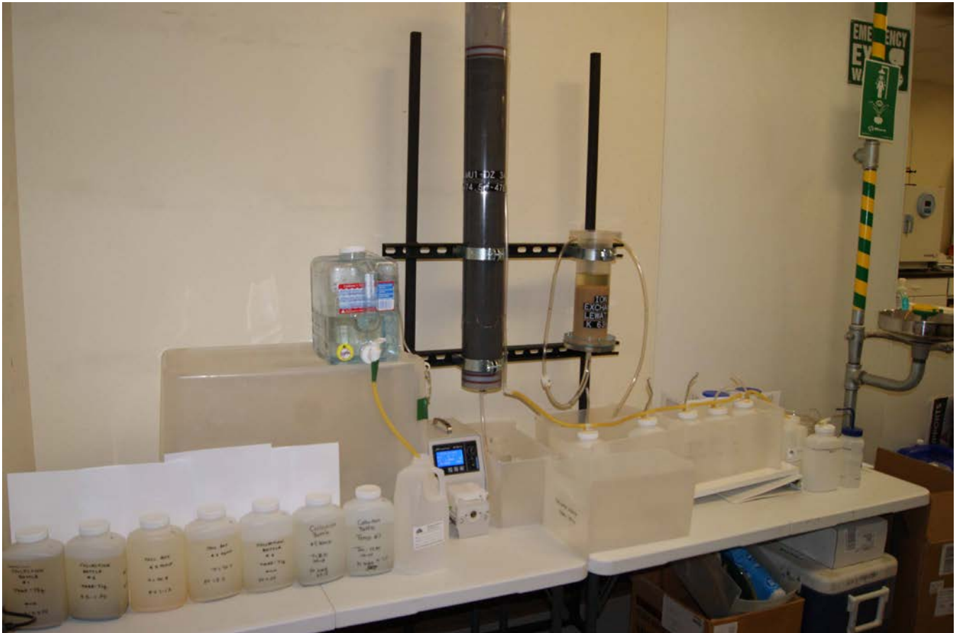
Figure 1: Low pH Column Leach Testing, Lance Projects, Wyoming USA
