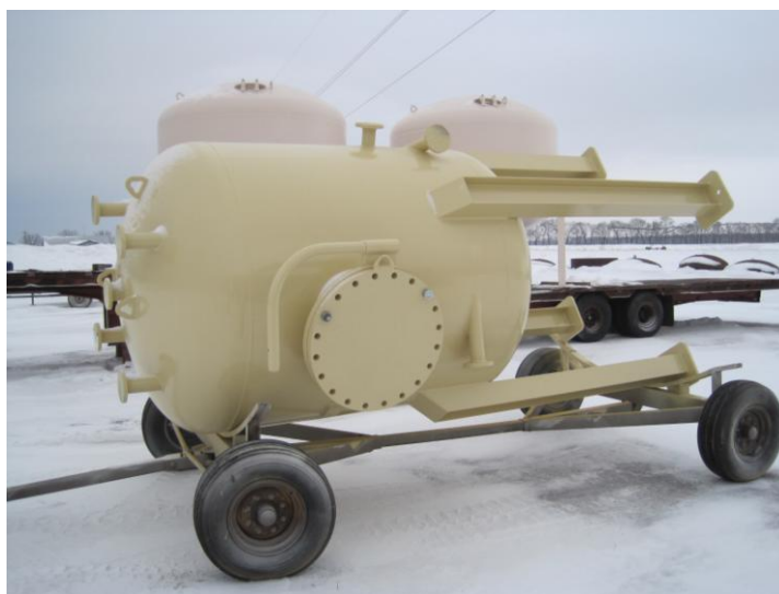
IMAGE 1.3 ION EXCHANGE COLUMN READY FOR INSTALLATION AT CENTRAL PROCESSING PLANT
